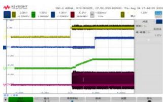
EN disable ,  $V_{\text{IN}}$ =12V , $V_{\text{OUT}}$ =1.0V,  $I_{\text{OUT}}$ =0A
