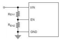
Figure 1: Undervoltage Lockout (UVLO) Voltage Divider Circuit
