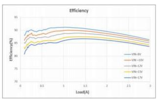
Output current vs. efficiency (Vout=5.05V)
