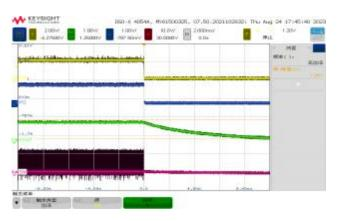
EN disable , V<sub>IN</sub>=12V ,V<sub>OUT</sub>=1.0V, I<sub>OUT</sub>=3A
