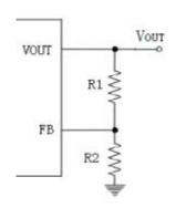
Figure 2: Voltage Divider Resistors for Setting the Output Voltage
