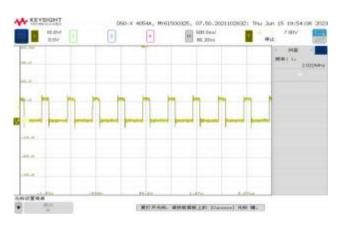
Switching frequency  $V_{\text{OUT}}=5V$  ,  $I_{\text{OUT}}=3A$
