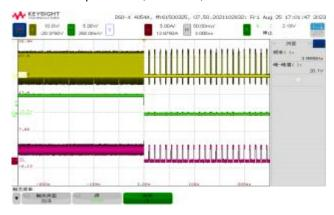
Short-circuit recovery, VIN=12V, VOUT=5V Short to 3A
