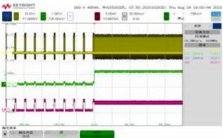
Short-circuit protection,  $V_{IN}$ =12V , $V_{OUT}$ =3.3V 3A to Short
