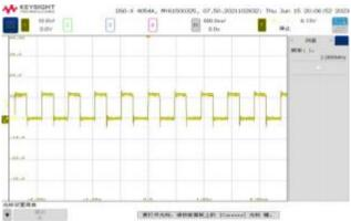
The test conditions are  $V_{IN}$  = 12V ,  $V_{OUT}$  = 1.0V, with external capacitors  $C_{IN}$ =2x10 $\mu$ F and  $C_{OUT}$  =  $2x47\mu$ F, and a temperature of TA = 25. C, unless otherwise noted.
