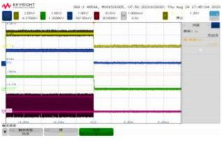
EN start ,  $V_{IN}$ =12V , $V_{OUT}$ =5V,  $I_{OUT}$ =0A
