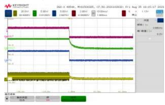
EN disable, V<sub>IN</sub>=12V, V<sub>OUT</sub>=5V, I<sub>OUT</sub>=3A
