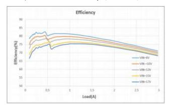
Output current vs. efficiency (Vout=3.25V)
