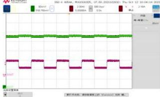
Load dynamic response ,  $V_{OUT} = 1V$  ,  $I_{OUT} = 0A -> 3A$
