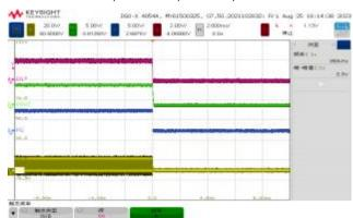
Short-circuit protection,  $V_{IN}=12V$ ,  $V_{OUT}=1.0V$  3A to Short
